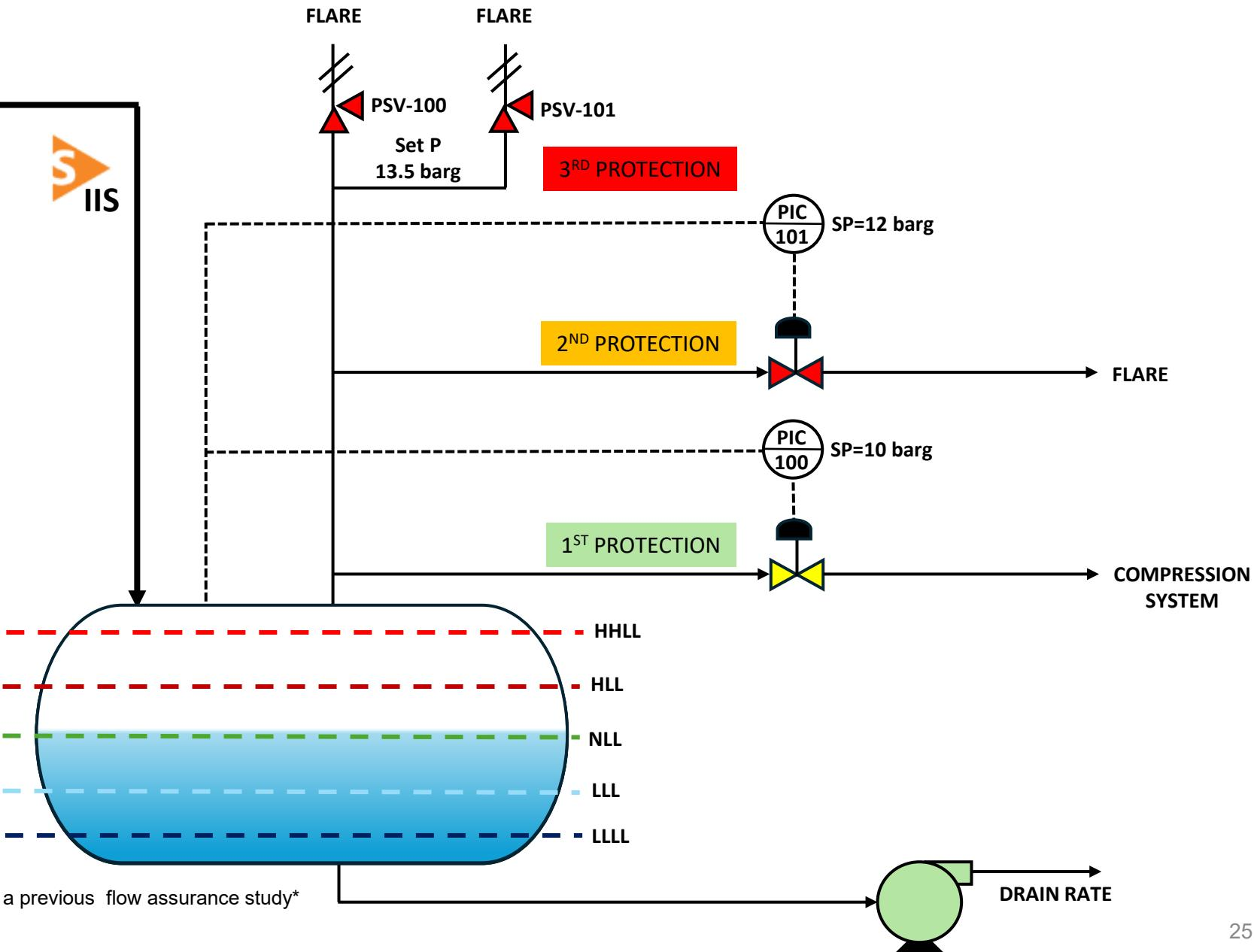
Only the drain rate was considered to size the Slug Catcher according to a previous flow assurance study\*
