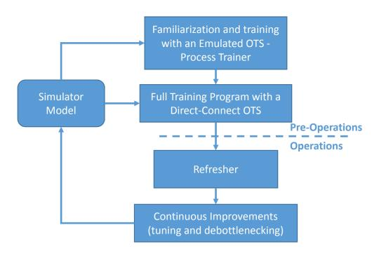
Yinson, in adherence to their Asset Integrity Management, needed an operators competency development plan, based on a high-fidelity simulator model, that should involve the pre-operation, operation and continuous improvements phases of the FPSO:
