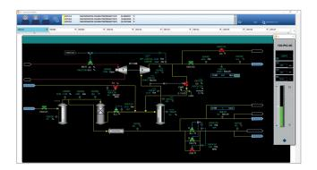
Additionally, the Operator Workstation has a powerful trending tool to recreate the same trendlines used in control room or to dynamically create specific trendlines for extra information from the historized data.
