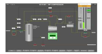
It allows to easily configure multiple windows, scroll bars, pull down menus, icons, push buttons, dialog boxes, embedded trends, customized faceplates... and connects them to data managed by the Communication Hub for any digital twin project or OTS. Furthermore, if some graphic files do exist, they can be embedded into the HMI being developed.
