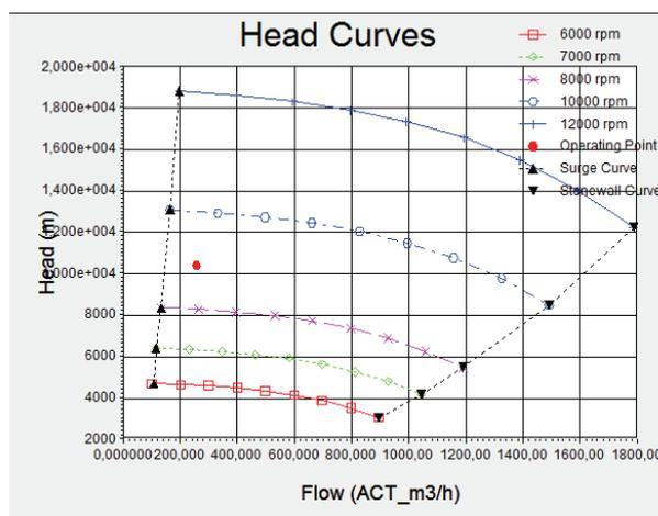
Figure 4. Example of a compressor map.
