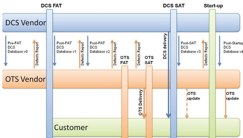
**Figure 5.** Revision cycles during an OTS implementation project.
