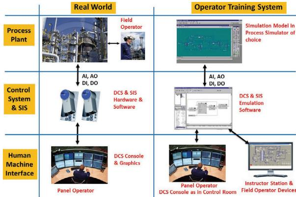
**Figure 1.** Elements of an operator training system and its equivalent in the real world.
